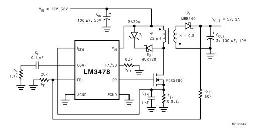
FIGURE 13. Typical Flyback Circuit
