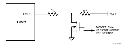
FIGURE 7. Shutdown Operation in Frequency Adjust Mode
