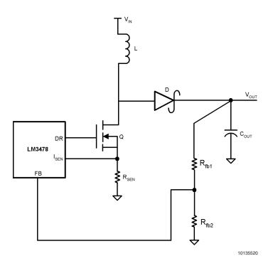
FIGURE 10. Adjusting the Output Voltage
