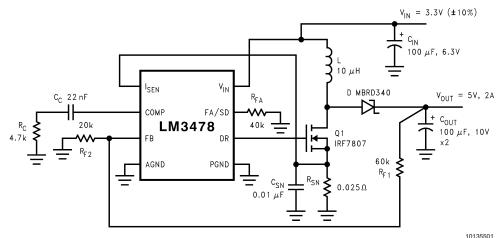
Typical High Efficiency Step-Up (Boost) Converter
