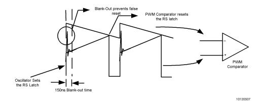
FIGURE 1. Basic Operation of the PWM comparator
