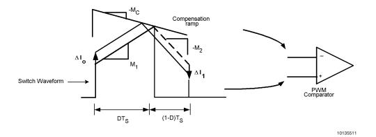
FIGURE 3. Compensation Ramp Avoids Sub-Harmonic Oscillation
