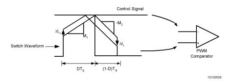
FIGURE 2. Sub-Harmonic Oscillation for D>0.5
