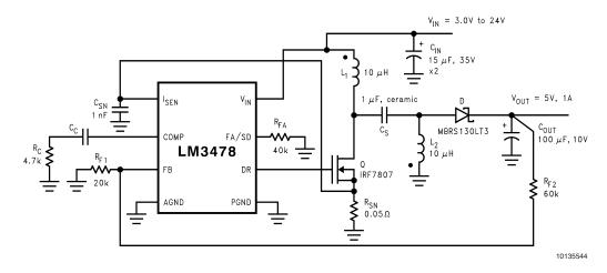
FIGURE 12. Typical SEPIC Converter
