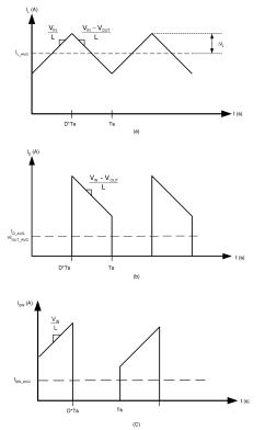
FIGURE 9. A. Inductor current B. Diode current
